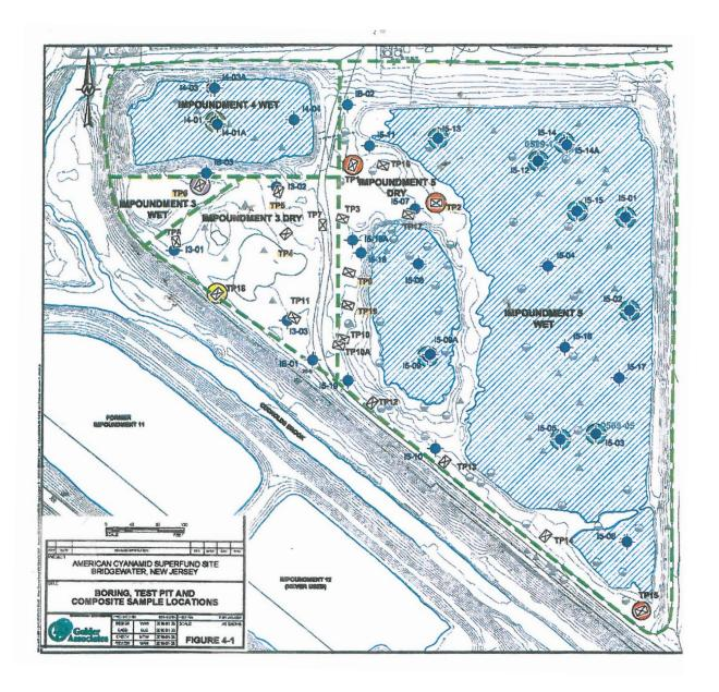
Historic reports were used to determine where borings and test pits for sampling should be located. Several geophysical methods, including marine geophysics were helpful in determining the extent of waste and debris. Air monitoring was conducted during test pit excavations to evaluate the emissions from open excavations to provide data for the design of future pilot study and full scale stabilization/solidification activities
